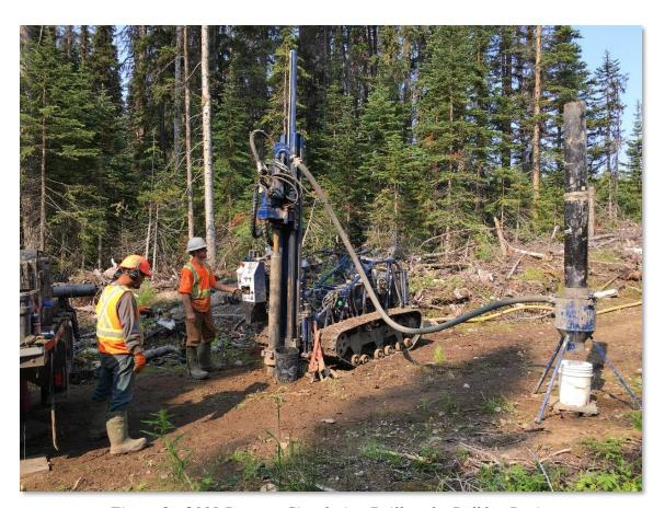
Figure 2 - 2019 Reverse Circulation Drill at the Bulkley Project
