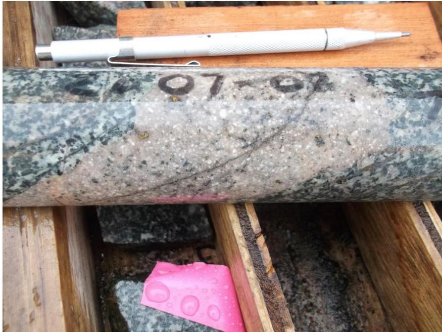
*Porphyry intrusion in DDH-2007-2 @ 77m associated with sheeted quartz-sulphide veining*
